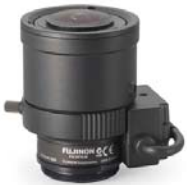
YV2.6x3C-SA2-L FUJINON 1/3" CS-mount Lens f=3.0~8mm/F1.4~ Close Aspherical - Auto Iris DC HVOF: 1/3"=95°~34°
