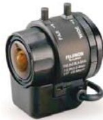
YV2.8x2.8LA-SA2-L FUJINON 1/3" CS-mount Lens f=2.8~8mm/F0.95~ Close Aspherical - Auto Iris DC HVOF: 1/3"=99°~34°
